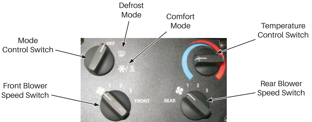
Figure 3-50. Single Overhead HVAC System
