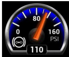
Figure 3-17. Brake Application Pressure
