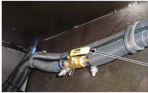
Figure 3-54. Heater Shut-off Valve Under Cab
