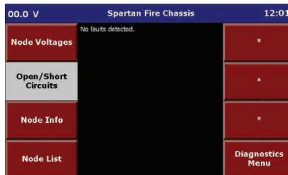
Figure 3-42. V-MUX Diagnostics Menu (Open/Short Circuits)
