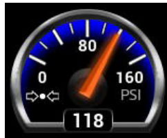
Figure 3-16. Auxiliary Air Pressure
