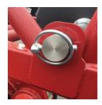
Figure 4-11. Rope Rescue Roller Assembly
