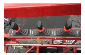
Figure 3-16. Ladder Tip Controls
