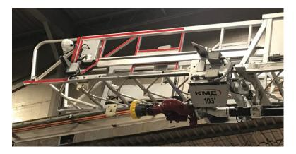
Figure 4-9. Monitor at the End of the Mid-Fly Section
