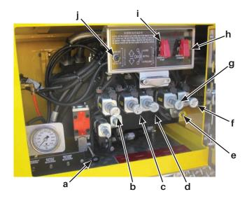
Figure 4-13. Diverter Valve Override & Stabilizer Manual Controls
