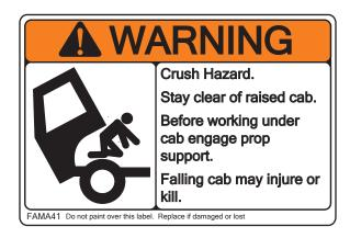
If the cab fails to lower after following the proper instructions, do not attempt to force it. Have the system checked by a qualified technician and refer to the cab tilt system instructions in the service manual.
