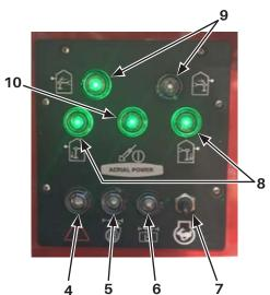
Figure 3-4. Stabilizer Controls - Direct Hydraulic
