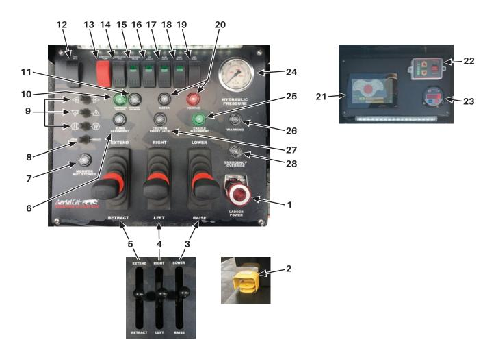
Figure 3-7. Primary Operator Control Station
