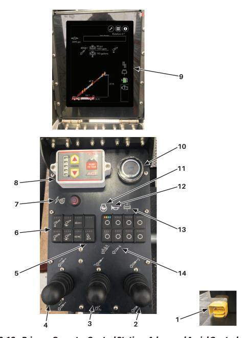
Figure 3-12. Primary Operator Control Station - Advanced Aerial Controls
