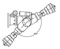
Figure 4-7. Nozzle motion - Extended Range
