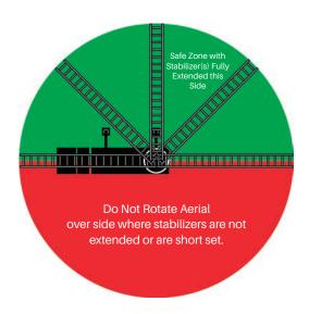
Figure 4-3. Short Set Rotation Interlock Stop Point
