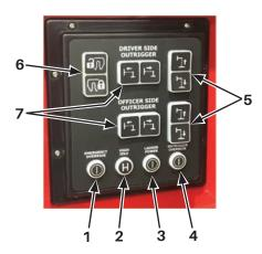
Figure 3-5. Stabilizer Control - Electric Over Hydraulic
