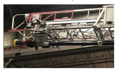
Figure 4-8. Monitor at the End of the Fly Section
