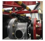
Figure 4-10. Aerial Standpipe Connection
