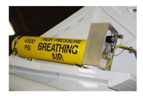
Figure 3-20. Breathing air system high-pressure cylinder
