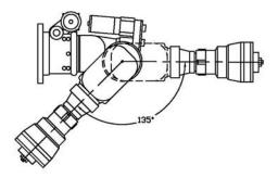
Figure 4-6. Nozzle motion - Standard Range
