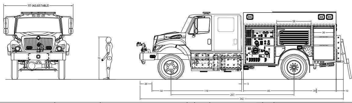
CAB: HV507 4X4 SFA 4 DR ENGINE & TRANS: CUMMINS L9 350 HP /ALLISON 3000 EVS AXLES: 14,000# FRONT/26,000# REAR
