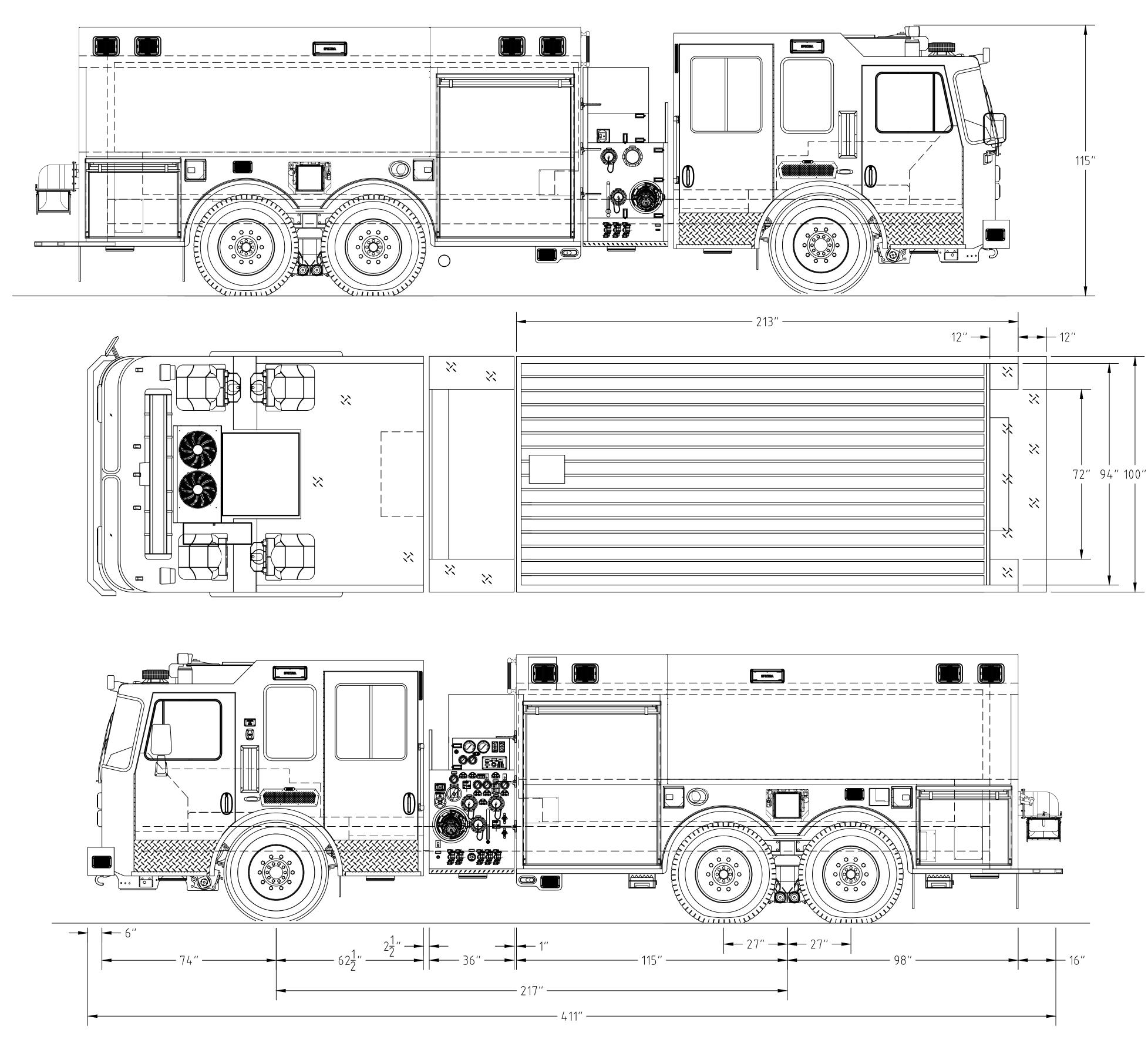
CAB: 100"W KME PANTHER MFD 10" RR ENGINE & TRANS: CUMMINS L9 450 HP/ 3000 EVS AXLES: 20,000# FRONT/48,000# REAR PUMP: HALE RSD - J 1000 GPM
