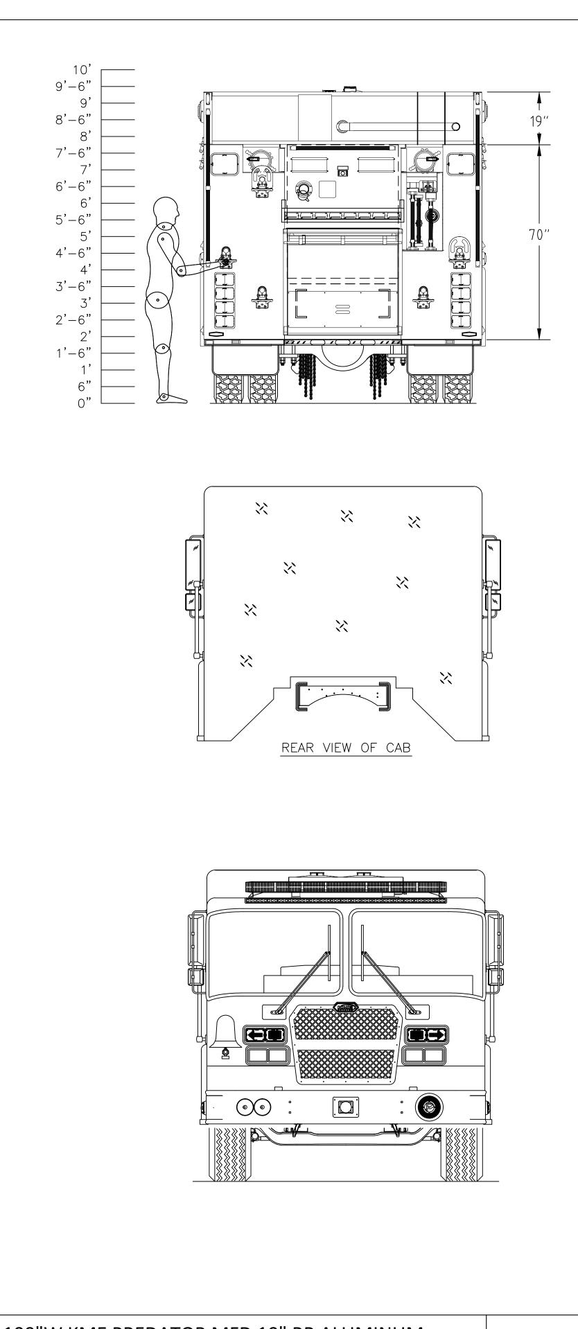
CAB: 100"W KME PREDATOR MFD 10" RR ALUMINUM ENGINE & TRANS: CUMMINS L9 450 HP/ALLISON 3000 EVS AXLES: 20,000# FRONT/27,000# REAR PUMP: WATEROUS CSU-C20 1,750 GPM SINGLE STAGE WATER TANK: 1,000 GALLONS POLY BODY TYPE: 158" PUMPER 3/16" ALUMINUM GENERATOR: HARRISON 6MCR PTO/HYD
