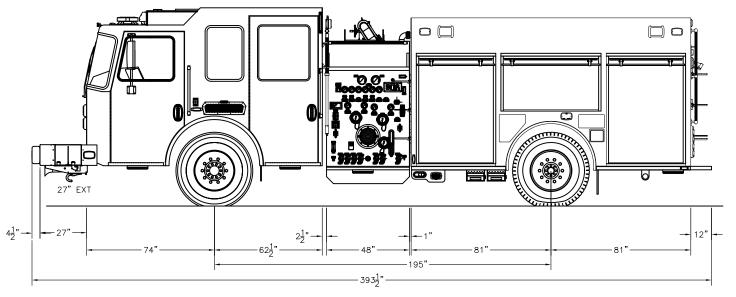
CAB: 100"W KME PANTHER MFD 10" RR VISTA ENGINE & TRANS: CUMMINS L9 450 HP/ALLISON 3000 EVS AXLES: 20,000# FRONT/27,000# REAR
