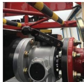
**Figure 4-10. Aerial Standpipe Connection**
