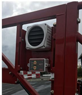
**Figure 3-15. Ladder Tip Communications System**
