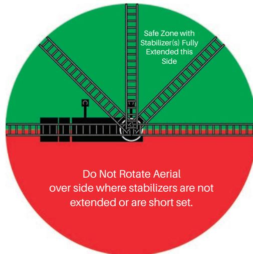
**Figure 2-2. Short Set Rotation Interlock Stop Points**
