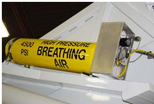
**Figure 3-20. Breathing air system high-pressure cylinder**
