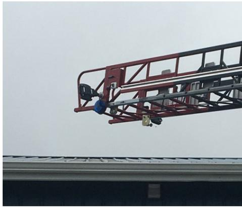
**Figure 4-5. Maintain sufficient ladder clearance**
