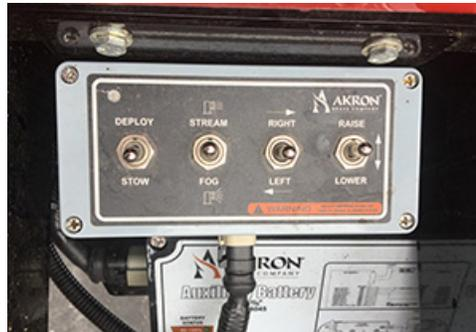
**Figure 3-17. Monitor Controls at Tip**
