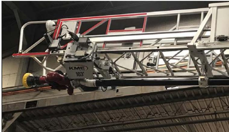
**Figure 4-8. Monitor at the End of the Fly Section**
