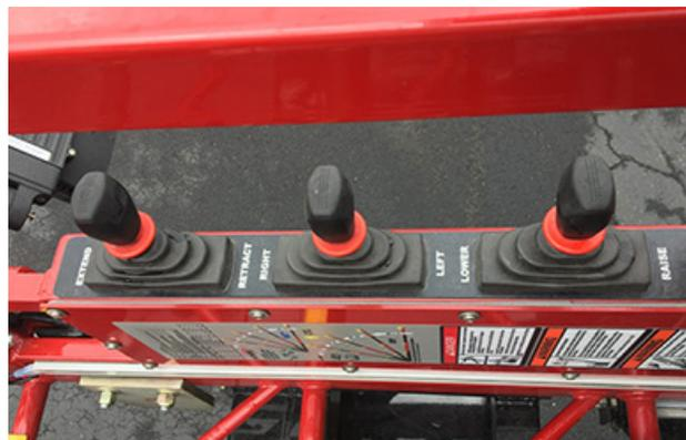
**Figure 3-16. Ladder Tip Controls**
