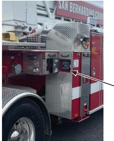
**Figure 3-3. Location of Stabilizer Control Panels - One on Each side of Trailer**
