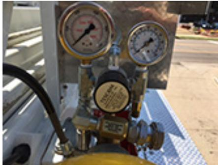
**Figure 3-21. Breathing air system gauges**
