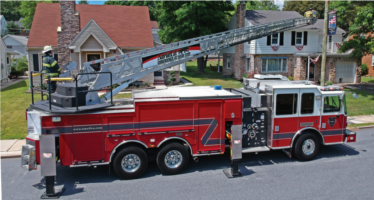
Short outrigger stance allows for setup on the tightest streets.
