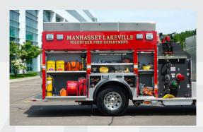
WITH FABRICATED BODIES CONSTRUCTED OF GALVANNEALED STEEL, ALUMINUM OR STAINLESS STEEL, KME PUMPERS PROVIDE ADDITIONAL COMPARTMENT SPACE TO CUSTOMIZE EQUIPMENT MOUNTING TO YOUR SPECIFIC NEEDS.
