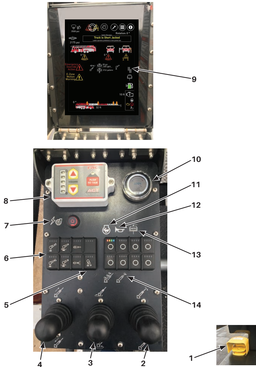
Figure 3-12. Primary Operator Control Station - Advanced Aerial Controls
