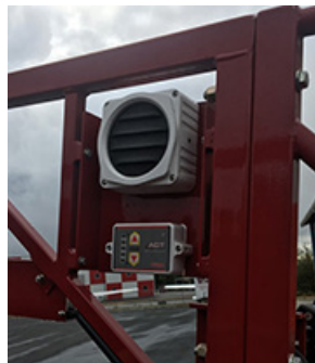
Figure 3-15. Ladder Tip Communications System
