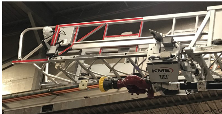
Figure 4-13. Monitor at the End of the Mid-Fly Section
