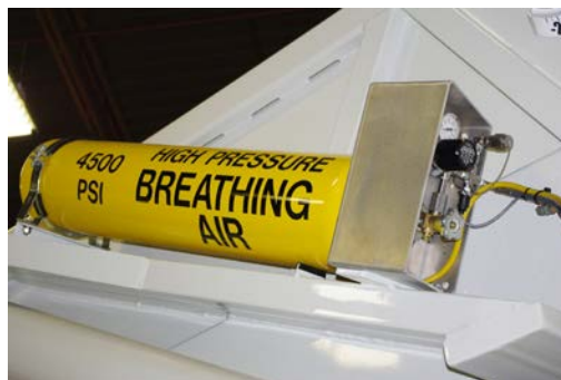
Figure 3-20. Breathing air system high-pressure cylinder
