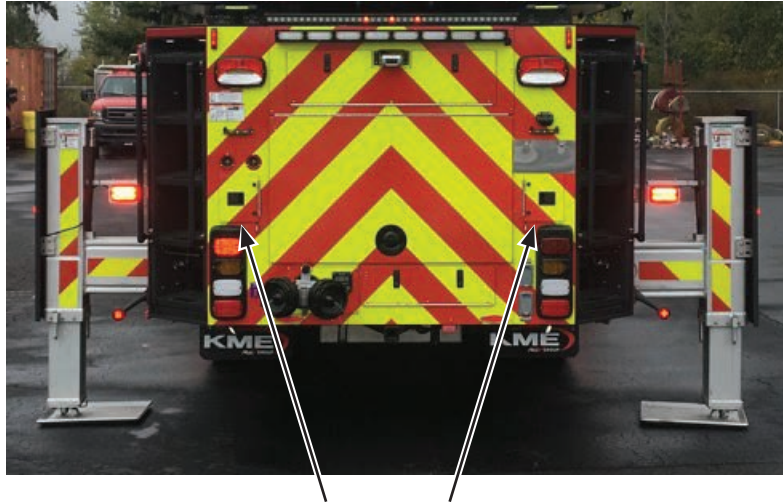
Figure 3-3. Location of Drivers Side and Passenger Side Stabilizer Control Panels
